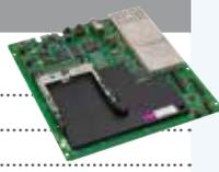
**QAM module** - Quad-QAM modulator, adjacent channel operation, automatic multiplexing, available as FTA or CI variant.
