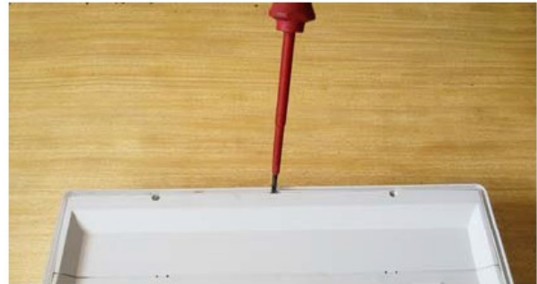
*disassemble the cover-reflector, prying with a screwdriver at the indicated point
