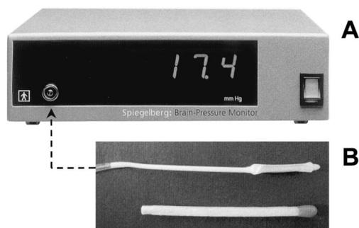
**FIGURE 1.** Photograph illustrating the tip of the Spiegelberg 3-PN sensor with the monitor (A) and the air pouch mechanism (B).
